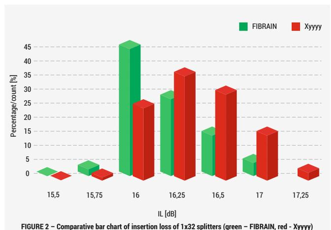
FIGURE 2 – Comparative bar chart of insertion loss of 1x32 splitters (green – FIBRAIN, red - Xyyyy)
