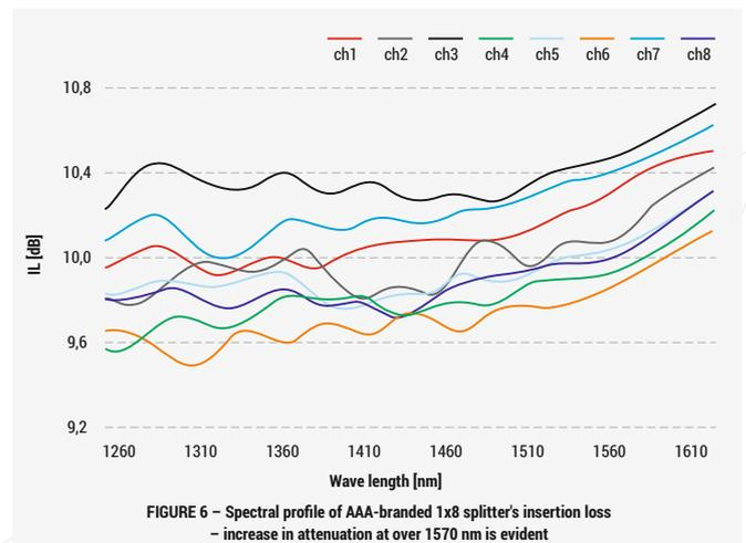
FIGURE 6 – Spectral profile of AAA-branded 1x8 splitter's insertion loss – increase in attenuation at over 1570 nm is evident
