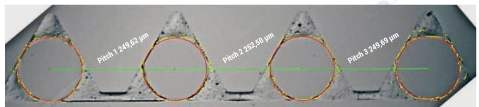
FIGURE 4 – Fiber array element extracted from Cccccc splitter – over 2 μm channels' misalignment is evident
