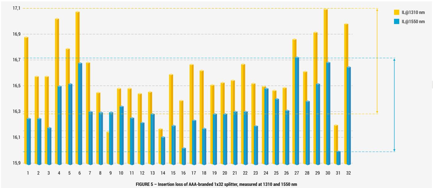
FIGURE 5 – Insertion loss of AAA-branded 1x32 splitter, measured at 1310 and 1550 nm
