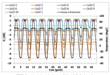
FIGURE 5 – Changes in insertion loss value for selected ports of AAA-branded 1x32 splitter during testing in the environmental chamber – fluctuations in attenuation value from 3 up to 9 dB
