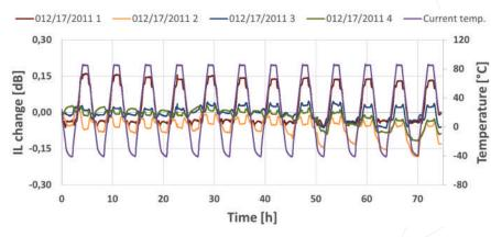
FIGURE 6 – Changes in insertion loss value for selected ports of Fibrain 1x8 splitter during testing in the environmental chamber
