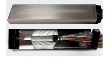
FIGURE 4 – Xyyyy-branded 1x32 splitter containing the insufficient amount of adhesive after testing in the environmental chamber.
