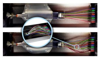
FIGURE 3 – Xyyyy-branded 1x32 splitter containing the correct amount of adhesive before (above) and after (below) testing in the environmental chamber. A receding fiber and macrobendings are evident.
