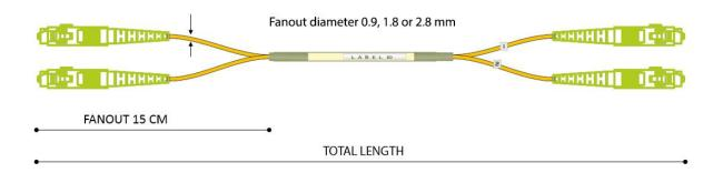
**PA4** – for cables terminated with two or four fiber optic connectors (for VC-DCY and AERO-DR03 also with a single connector), metal spring tube 3.0 mm made of stainless steel covers and protects fanouts at their whole length from the furcation point to the connector, providing 2000 N crush resistance. Cables: *VC-D20, VC-D40, VC-40R, VC-D40RP 2F, VC-DCY 2-4F, VC D20E 2-4F, VC-D30E 2-4F, VC-D40E 2-4F, AERO-DR03 1-2F*
