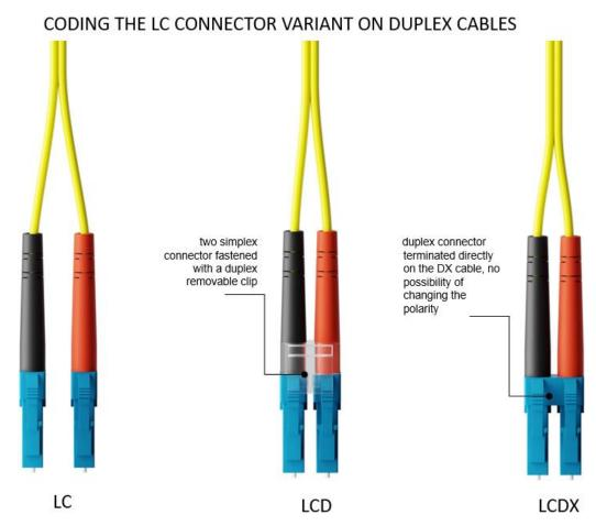
LC duplex patch cords are produce with AB polarity type as a standard. For AA type please add description on the order.
