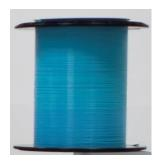
The fiber's Brillouin gain profile was designed for high accuracy distributed strain sensing applications. Scattering peak parameters that assure optimal sensor operation are Brillouin frequency shift > 10.850 GHz and Brillouin bandwidth < 35 MHz. The central frequency can be adjusted according to Customer's order. Cladding diameter and refractive index are equal to standard telecom fiber parameters
