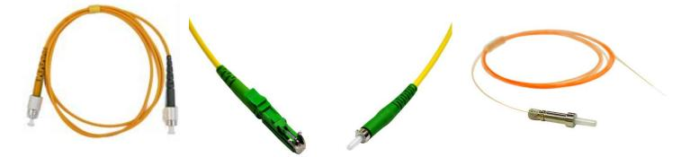
Thermally expanded core termination is used to ease coupling between fiber and free space. Core thermal expansion allows coupling beams with higher mode field diameter and numerical aperture to the standard single mode fiber. The terminations are available as patchcords with connectors, patchcords with connector and ferrule (TEC side) or as pigtails with a ferrule on the TEC side.
