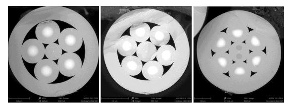
Multi-mode combiners are passive devices that allow coupling light from a few multimode laser sources into one fiber and are commonly used in high power optical lasers and amplifiers. Fibrain combiners are characterized by high pump efficiency (min. 90%) and low insertion loss (max. 0.5 dB).
