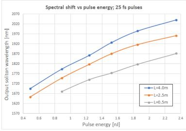
Typical wavelength-tuning characteristics, dependence on the input pulse energy, 50 fs input pulses, for 3 different nonlinear fiber lengths:
